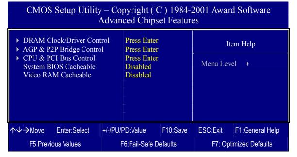
After you have completed the changes, press [Esc] and follow the instructions on your screen to save your settings or exit without saving. The following table describes each field in the Advanced Chipset Features Menu and how to configure each parameter.
