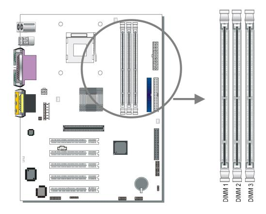
Your board comes with three DIMM sockets, Directly supports one SDR SDRAM channel, 64b wide, providing support max of 3 Double-Sided DIMMs with unbuffered PC133. *The largest memory capacity possible is 3GB*. On this motherboard, DRAM speed can be set independent from the CPU front side bus speed. Depending on the DRAM clock speed setting in the BIOS setup.
