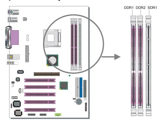
The P4VGA mainboard supports non ECC and non registered DDR and SDRAM modules.
