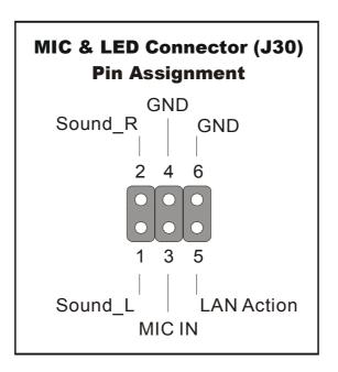
You can connect the Line-out /MIC in/LAN LED to the front panel of your PC case. (If this option is available in your PC case.)
