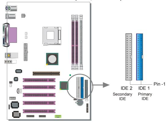
This Motherboard offers two primary and secondary IDE device connectors (IDE1, IDE2). It can support up to four high-speed Ultra DMA 33/66/100/133 HDD or CD-ROM.
