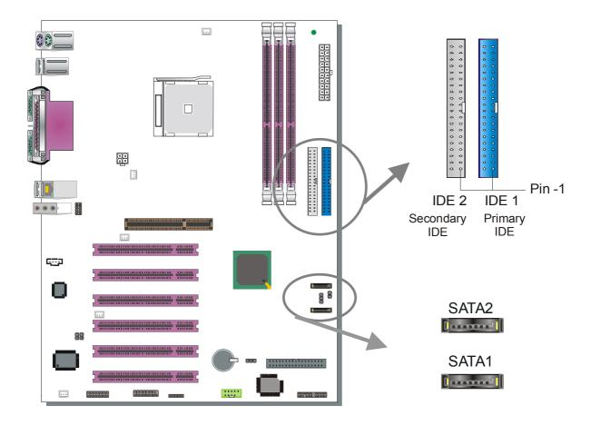
This Motherboard offers two IDE connectors (IDE1, IDE2) and 2 serial ATA ports. IDE1 and IDE2 can support up to four high-speed Ultra DMA 33/66/100/133 HDD or CD-ROM. SATA1 and SATA2 can support up to two 150 SATA hard disks. This Motherboard can support up to 6 HDDs.
