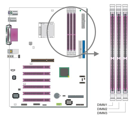
Your board comes with three DIMM sockets, providing support for up to 3GB of main memory. On this motherboard, DRAM speed can be set independent from the CPU FSB speed.
