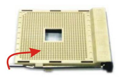
2. Align the blunt edge of the CPU with the matching pinhole distinctive edge on the socket.
