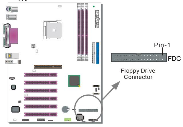
The system supports 5 possible floppy drive types: 720 KB, 1.2 MB, 1.44 MB, 2.88 MB. In addition, this Motherboard supports a 3-mode (720KB/1.2MB/1.44MB) floppy commonly used in Japan.
