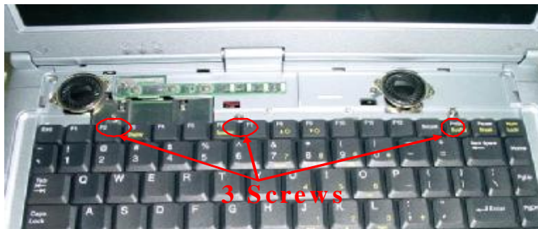
Figure 2-4 Remove Three Screws on the Keyboard
