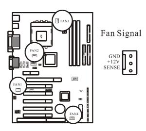
■ FAN3: CPU Main FAN , FAN2: CPU Secondary FAN
