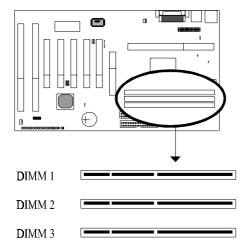
Insert the module as shown. Due to different number of pins on either side of the breaks, the module will only fit in the orientation as shown. There is no jumper setting for memory configuration.
