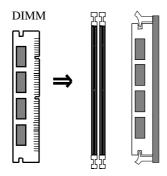
Chipset only allows synchronuos operation for DIMM and CPU. Therefore, the system must install 100 MHz "PC-100 SDRAM memory DIMM" (3.3V) for 100 MHz Deschutes CPUs. For 66 MHz Celeron<sup>TM</sup> CPUs, the user may use either 3.3V EDO RAM or SDRAM.
