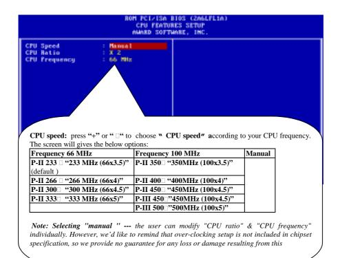
Since this is a jumperless design, there is no jumper setting to adjust CPU speed. The user only needs to set speed in BIOS. Enter BIOS, find "CPU speed" under "Chipset Features Setup," and set as above.
