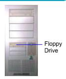
**2.** Place the drive from the front panel side into the frame.
