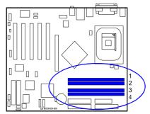
**2.** Install DDR DIMM straight down into the socket 1 using both hands, then socket 2, and so forth.
