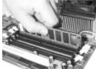
3. The clip on both ends of the socket will close up to hold the DDR DIMM in place when the DDR DIMM reaches the socket bottom.
