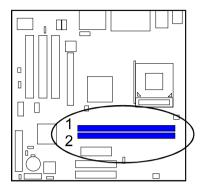
Press the clips with both hands to remove the DIMM.
