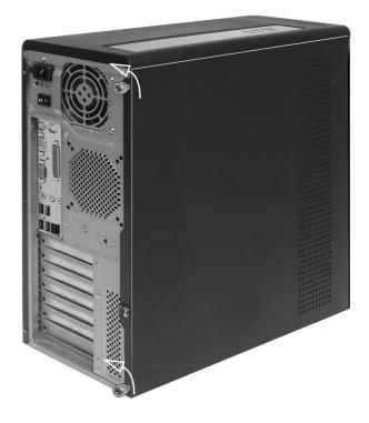
4 Hold right panel(from rear view) with both hands. Slide it back about an inch and then gently pull it outward to detach it.
