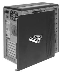
2 Secure the side panels with the two thumbscrews.
