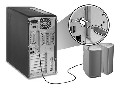
audio line-in device: connects to the Audio-in/Line-in jack ((\*))
