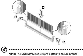
**Note:** The DDR DIMM sockets are slotted to ensure proper installation. If you insert a DDR DIMM but it does not fit easily into the socket, turn the DDR DIMM around and try to insert it again.
