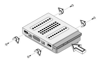
8. Reinstall the hard disk frame into the housing (see figures below).
