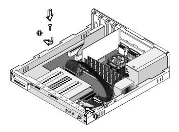
9. Reinstall the drive frame into the housing (see figures below). Make sure the tabs on both sides snap into place.
