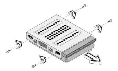
7. Insert the new hard disk into the hard disk frame and secure it with the four screws.
