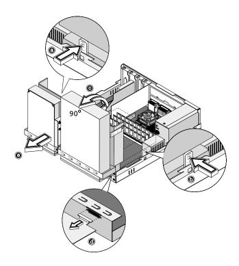
4. Detach hard disk cable (a) and power cable (b) from the hard disk. Then, remove the screw that holds the hard disk to the housing (c). Set the screw aside.
