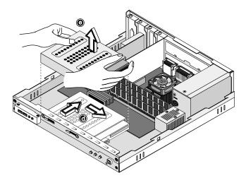
6. Remove the four screws that hold the hard disk to the hard disk frame and detach the hard disk. Set the screws aside.
