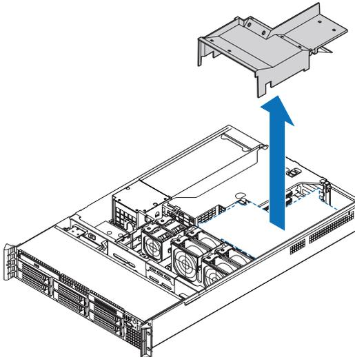
To install the CPU air duct:
