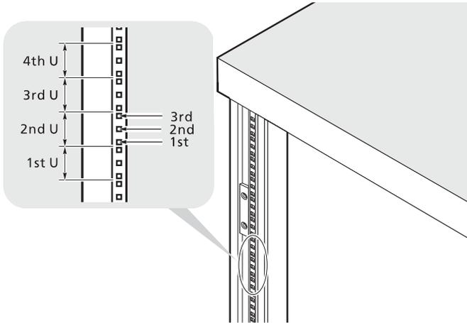
The system occupies 2U in the rack. Count the U positions and hole numbers from the bottom up.
