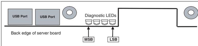
The following table lists the possible POST codes that may be displayed on the Diagnostic POST code LEDs during system initialization.
