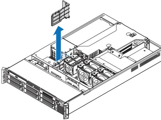
To install the small air baffle:
