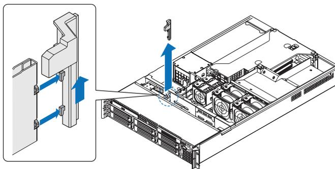
To remove the large air baffle:
