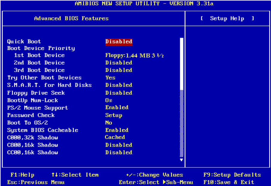
Figure 4-4A. Advanced BIOS Features Setup Menu Upper Screen Shot
