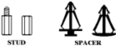
Figure 3-3. The outline of stud and spacer
