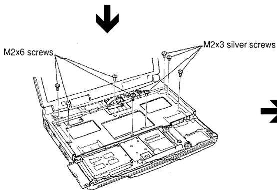
To remove the top cover with display assembly, follow the steps below.
