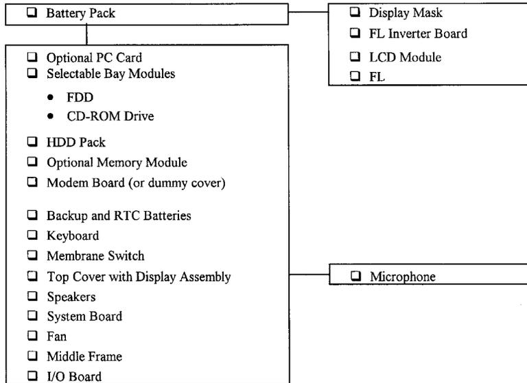
This section explains how to remove Field Replaceable Units (FRUs). It may not be necessary to remove all the FRUs in order to replace one.
