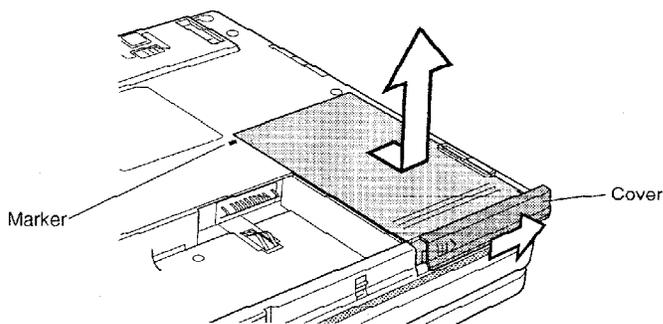
**CAUTION:** Be very careful not to press on the top or bottom of the HDD. Pressure can destroy data or damage the drive.
