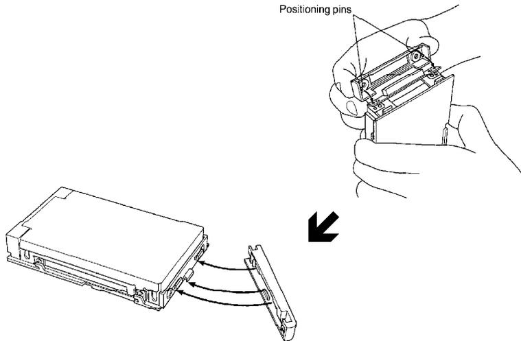
To assemble the HDD pack, follow the steps below.
