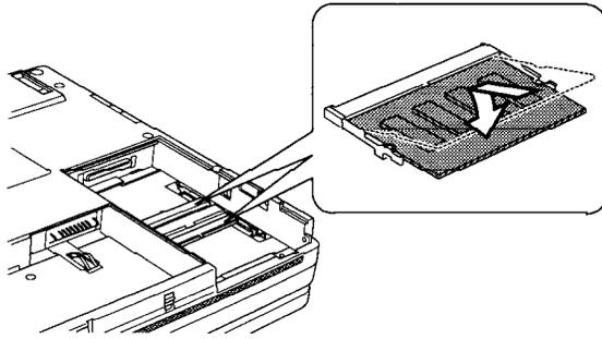
To install a memory module(s), make sure the computer is in boot mode and follow the steps below.
