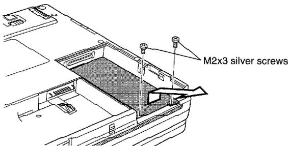
To remove the memory module(s), make sure the computer is in boot mode and follow the steps below.
