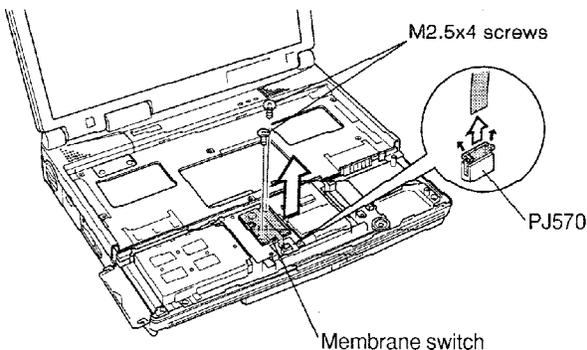
To remove the membrane switch, follow the steps below.
