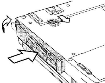
To remove the optional PC card, make sure the computer is in boot mode, then follow the steps below.
