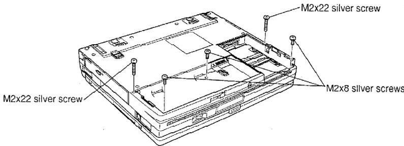
The modem board is located under the palmrest. To open the palmrest, follow the steps below.
