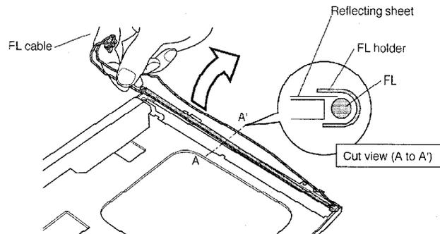
**CAUTION:** When you remove the **FL**, be careful not to let any dust or other foreign matter contaminate the **LCD panel**. Any contamination can affect the performance of the unit.
