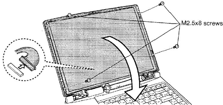
**NOTE:** Be careful not to apply pressure to the ICs along the edge of the LCD module. The ICs are easily damaged.
