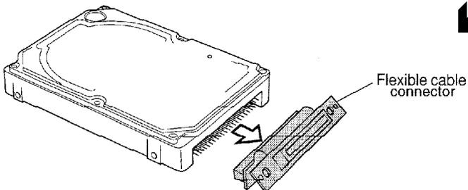
To disassemble the HDD Pack, follow the steps below.
