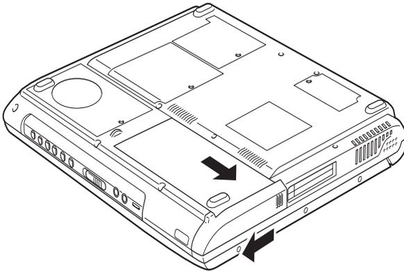
*Sliding the battery release latch*
