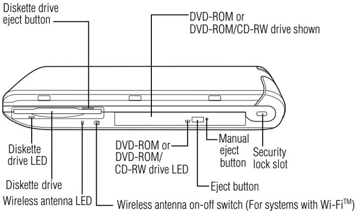
The **diskette drive LED** (light-emitting diode) glows when the diskette drive is in use.
