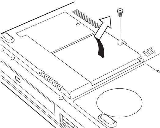
*Removing the expansion memory slot cover screw*
