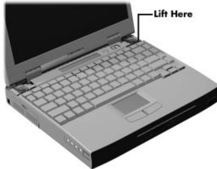
**Figure 4-9 Lifting Up the Keyboard**
