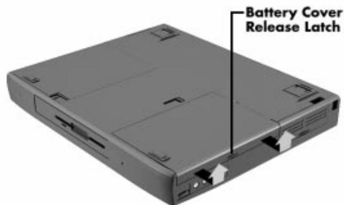
*Figure 2-5 Removing the Cover*
