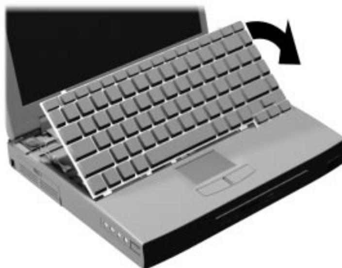
*Figure 2-16 Positioning the Keyboard*
