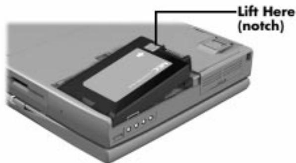
**Figure 4-6 Removing the Battery**
