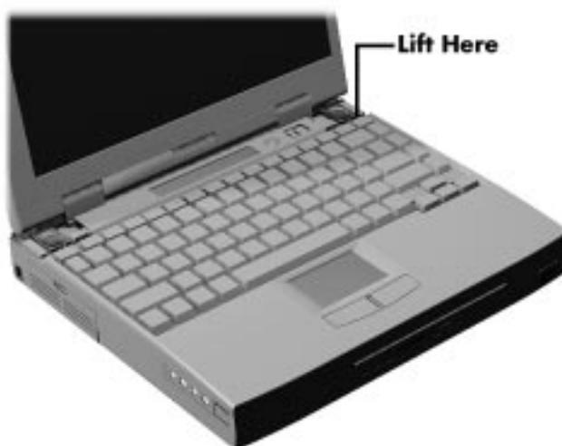
*Figure 2-15 Lifting the Keyboard*
