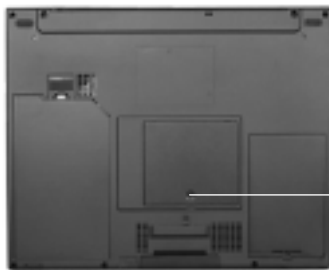
Removing the memory bay door
