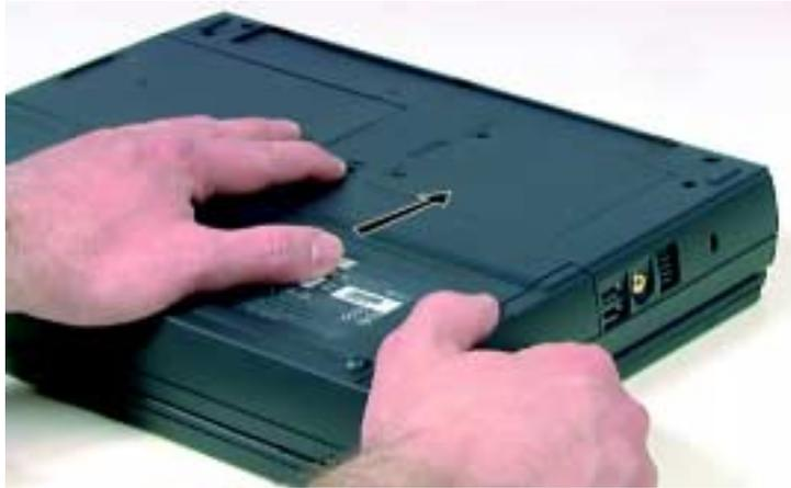
5. Hold the latch forward and slide the battery pack straight out from the notebook.
