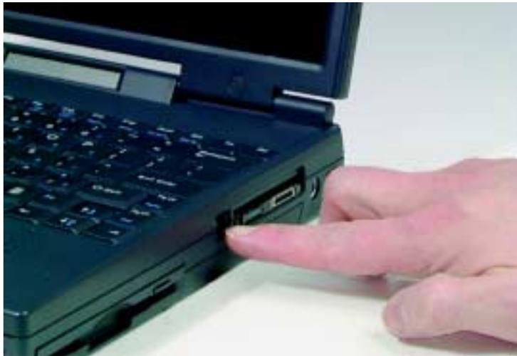
6. Press the PC Card eject button a second time to eject the PC Card.
