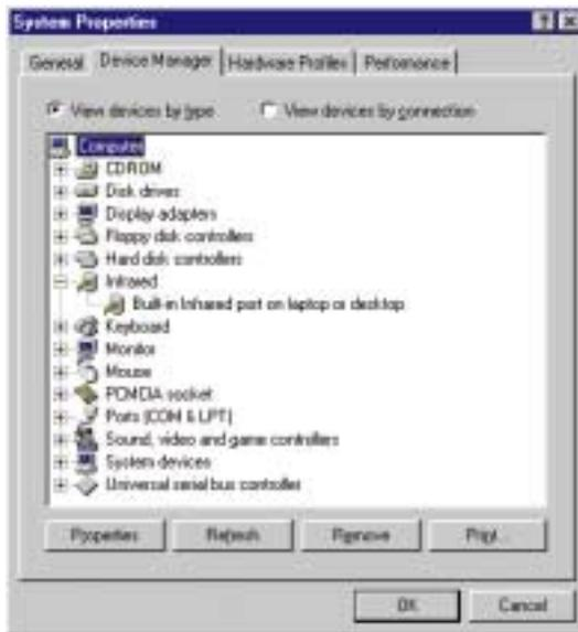
6. Double-click **Built-in Infrared port on laptop or desktop**. The **Built-in Infrared port on laptop or desktop Properties** dialog box opens.
