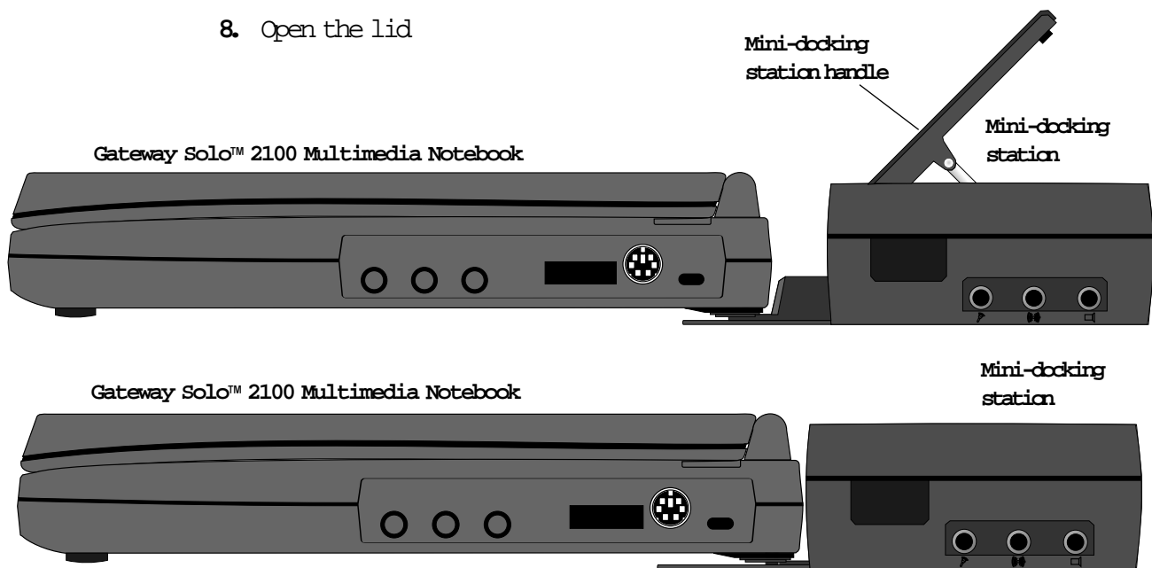
Figure 40. Connecting the Mini-Docking Station
