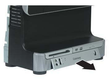
**4** Remove the two screws that secure the speaker grille panel to the computer.
