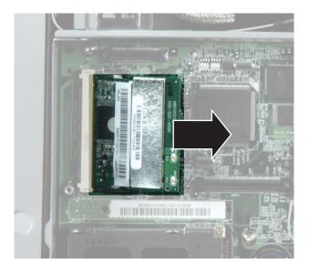
Insert the new Mini PCI card into the slot, then press it down until the retaining clips snap into place. The card must be fully seated in the slot before the retaining clips will snap into place.
