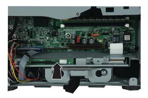
From the front of the computer, pull the drive out of the computer.
