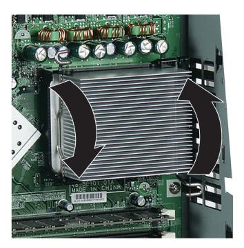
**5** Gently move the heat sink side to side to loosen it from the processor, then lift the heat sink away from the processor.
