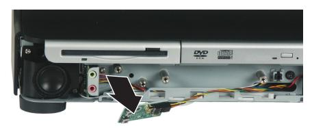
**8** Remove the two screws from the speaker you are replacing.
