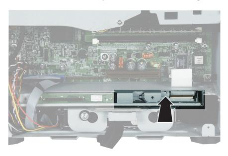
**7** From the front of the computer, pull the drive out of the computer.
