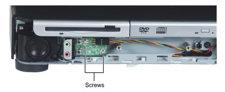
**7** Pull the front control circuit board away from the computer to expose the left speaker wires that run underneath it.
