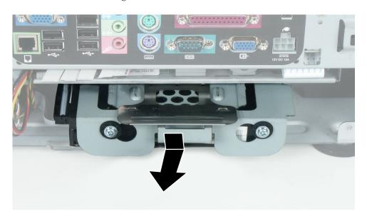
**4** While holding the latch, pull the drive cage out of the computer.
