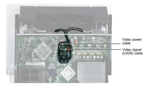
Thread the two video cables through the hole at the top center of the chassis.
