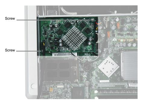
**5** Pry under the lower-right corner of the board to pull it loose, then pull the entire video board away from the computer.
