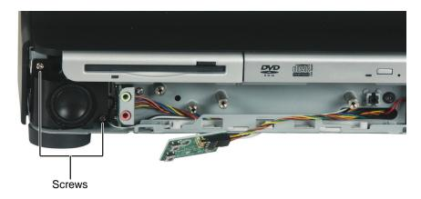
**9** Pull the speaker out of the computer while carefully threading the speaker wire out of the wire access port.
