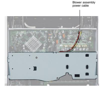
**4** Remove the three screws that secure the blower assembly to the computer.
