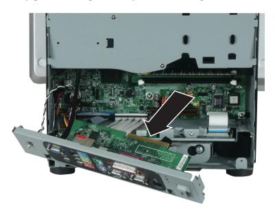
**5** Unplug the intrusion switch cable and other cables that connect the I/O panel to the computer.
