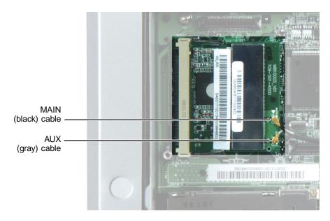
Press outward on the two Mini PCI retaining clips until the card flips up.
