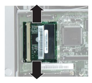
Remove the Mini PCI card from the slot.
