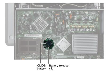
**5** Press the new CMOS battery into place.
