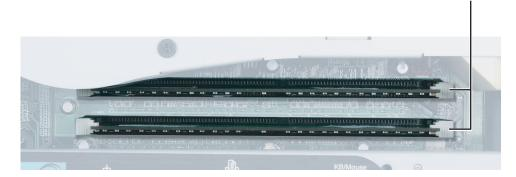
**3** If you are removing a memory module from the memory module bank, gently pull the plastic tabs away from the sides of the memory module and remove it.
