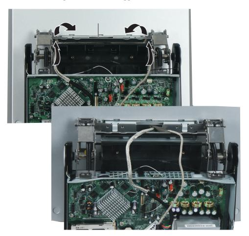
**12** Slide the LCD panel all the way up again, then remove the four screws that secure the hinge to the LCD panel.
