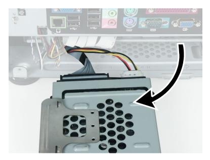
**5** Disconnect the drive cable and power cable from the hard drive.
