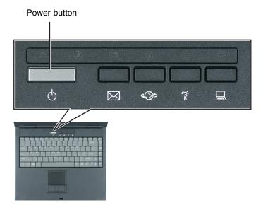
The power button is preset to On/Off mode. However, you can also set it to function in Standby/Resume mode. For instructions on changing the power button mode, see "Changing power settings" on page 147.
