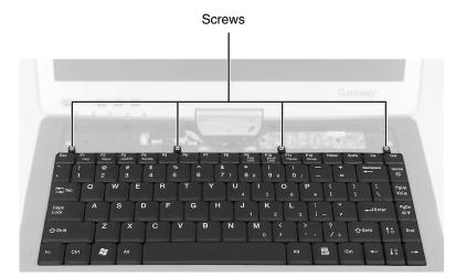
**13** Lift the back edge of the keyboard, then slowly rotate it toward you so it lies **keys-down** on top of your convertible tablet PC. Be careful not to damage the LCD panel.
