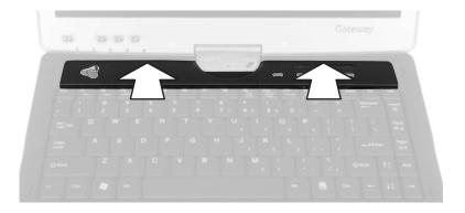
10 Press down on the bezel in several places to make sure it is correctly mounted. The bezel is correctly mounted when you can run your finger along the bezel and find no loose spots. The bezel should be flat all the way across.
