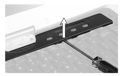
11 Remove the bezel from your convertible tablet PC by pulling the bezel toward you and at the same time lifting its front to clear the keyboard. You will hear small snapping sounds as the bezel comes away from your convertible tablet PC. Be careful not to break off the tabs found on the bottom of the bezel.
