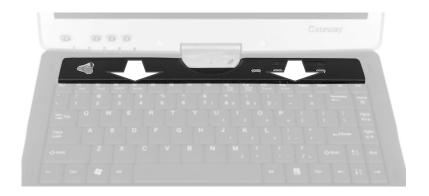
**12** With a small Phillips screwdriver, remove the four keyboard screws and put them in a safe place.
