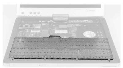
**14** Carefully insert the small flat-blade screwdriver between the keyboard cable and the black plastic hinge where the cable connects to the system board. Gently lift the hinge off the cable. The cable is now free and you can remove the keyboard.
