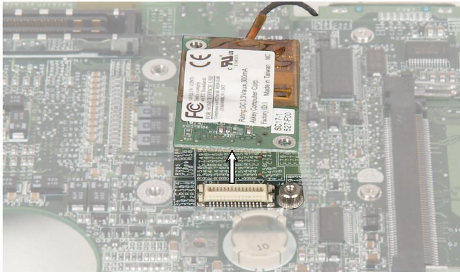
**28** Unplug the modem cable from the modem.
