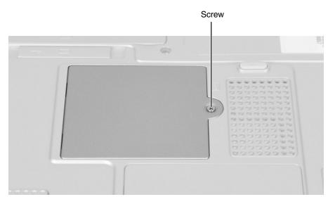
**5** Tilt the screw side of the cover upward.
