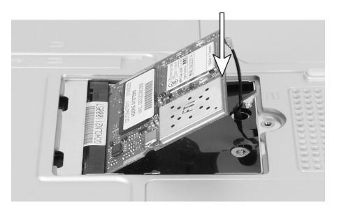
**12** Reattach the antenna cables to the card connectors.
