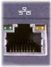
If you ordered the optional integrated network adapter, use this connector to connect the computer to a network.
