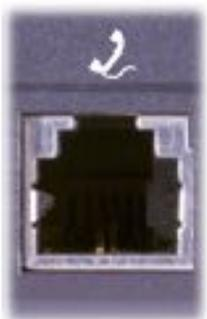
If you ordered the optional internal modem, use this connector to plug in the telephone connector.
