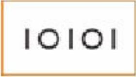
Use this connector to attach a serial device to the computer.
