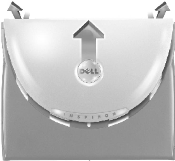
4. To replace the display cover, bend it slightly to insert the four tabs on the rounded edge of the cover into the slots on the top of the computer.
