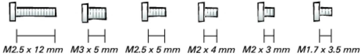
**NOTICE:** When reinstalling a screw, you must use a screw of the correct diameter and length. Make sure that the screw is properly aligned with its corresponding hole, and avoid over tightening.
