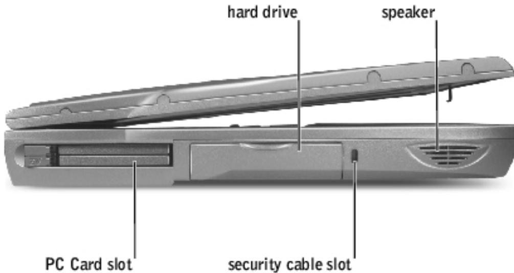
**PC Card Slot** — Has two connectors that support various types of PC Cards, including modems and network adapters. For more information, see the *Tell Me How* help file (see "[Accessing Help](#)").
