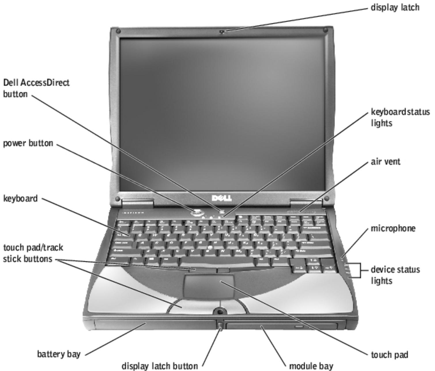
**Display Latch** — Keeps the display closed.
