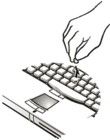
2. Align a new cap over the square track stick post and gently press the cap down onto the post.
