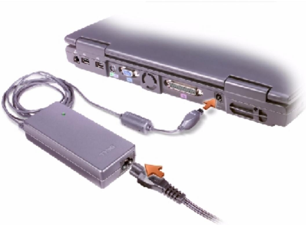
**⚠ CAUTION:** The AC adapter works with electrical outlets worldwide. However, power connectors and power strips vary among countries. Using an incompatible cable or improperly connecting the cable to the power strip or electrical outlet may cause fire or equipment damage.
