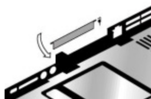
Figure 2-21. Removing a PCMCIA Door
