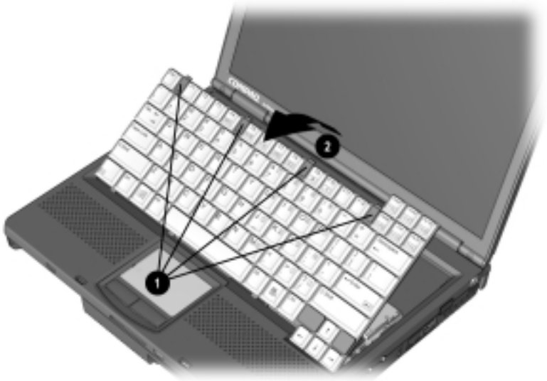
Figure 5-8. Releasing the Keyboard
