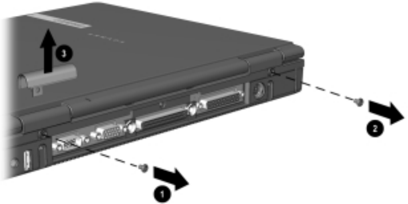
Figure 5-12. Removing the Switch and Hinge Cover Screws
