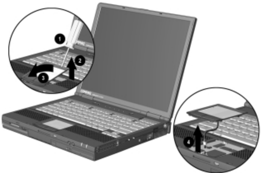
Figure 5-5. Removing the Touch Button
