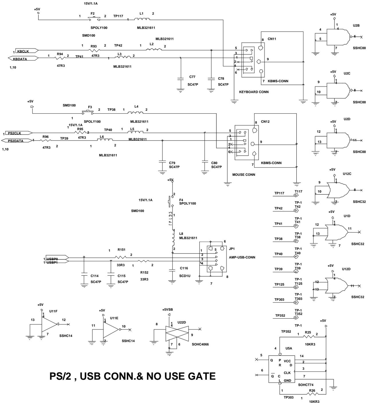
**Figure B-3 MPB Main Board (Motherboard) Logic Diagrams (Sheet 9 of 10)**
