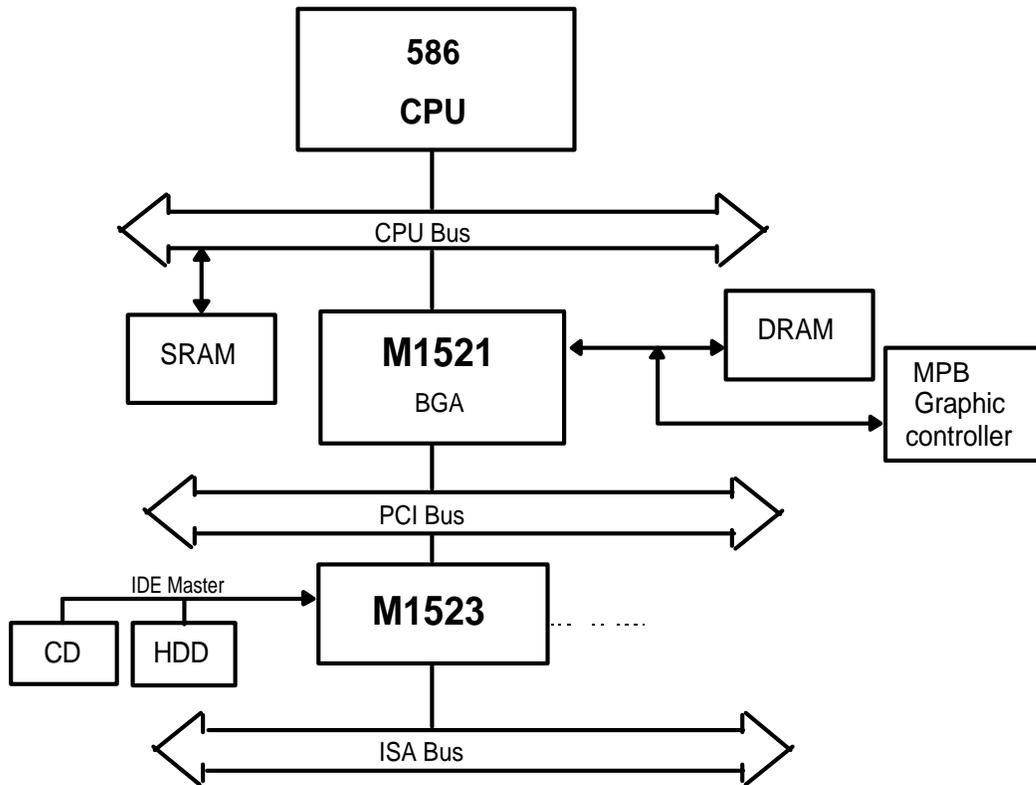
**Figure 4-1 Extensa Functional Block Diagram**
