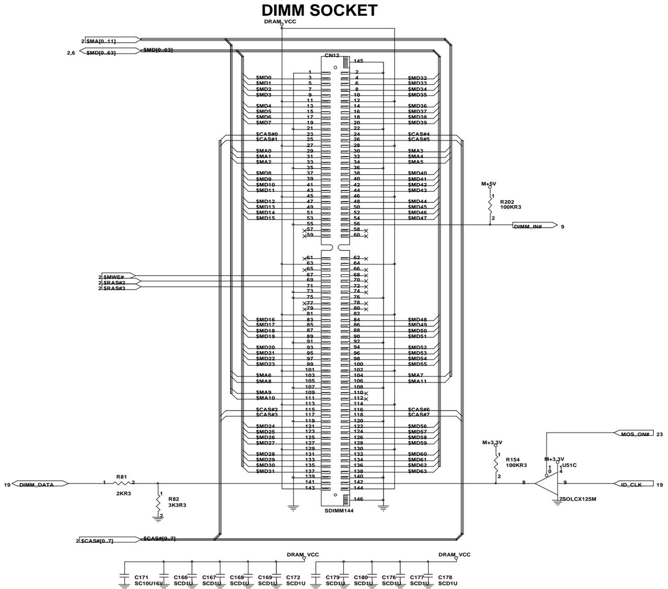
**Figure A-1 Notebook Main Board Logic Diagrams (Sheet 7 of 30)**
