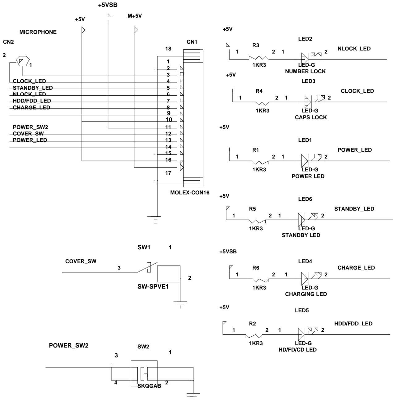
Figure B-6 MPB LED Board Logic Diagrams (Sheet 1 of 1)
