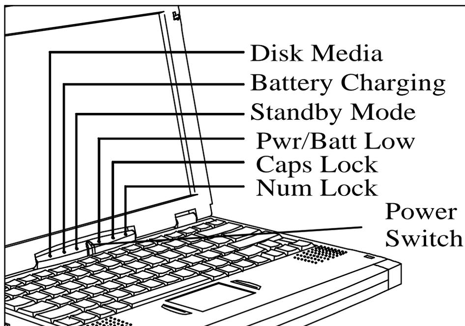
**Figure 3-1 Operating Controls and Indicators**
