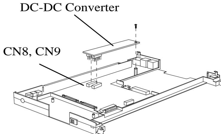
**Figure 6-30 Removing/Replacing the MPB DC-DC Converter Board**
