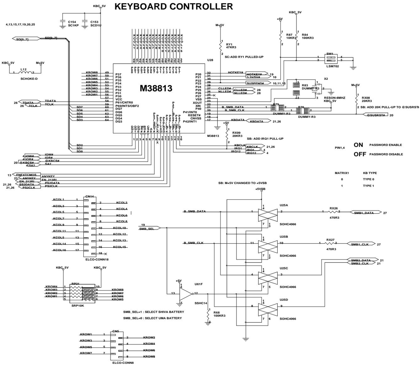
**Figure A-1 Notebook Main Board Logic Diagrams (Sheet 14 of 30)**
