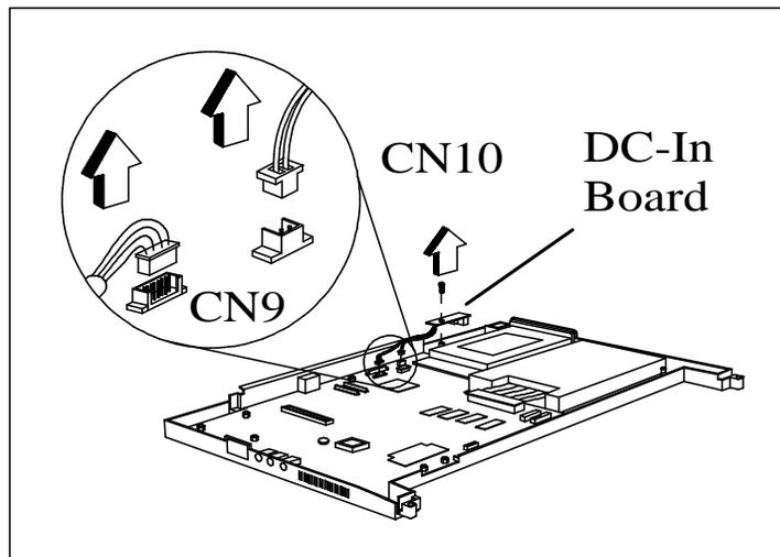
**Figure 6-18 Removing/Replacing the DC-In Board Assembly**
