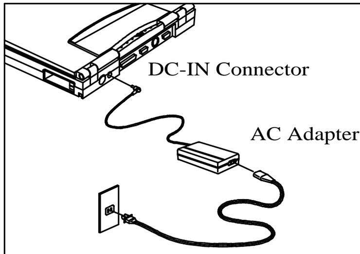
**Figure 2-11 Installing the AC Adapter**
