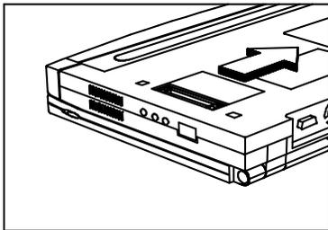
② Slide release latch on MPB forward; swing the docking level outward 90 degrees
