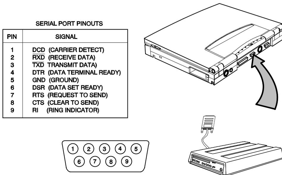
**Figure 2-8 Serial Port Pinouts**
