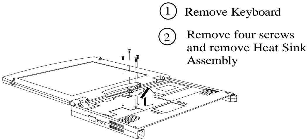
**Figure 6-11 Heat Sink Assembly Removal/Replacement**
