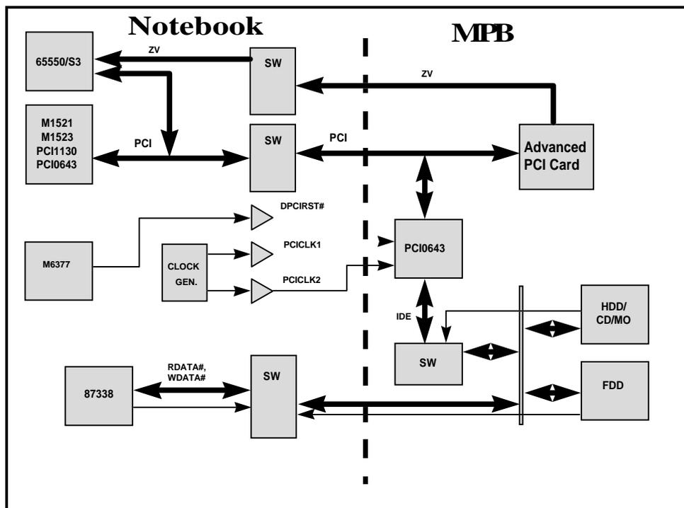
Figure 4-5 MPB Interface Diagram
