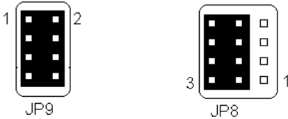
CPU Power Setting for Intel Pentium CPU (3.5V) or Cyrix 6x86 or AMD-K5 CPU
