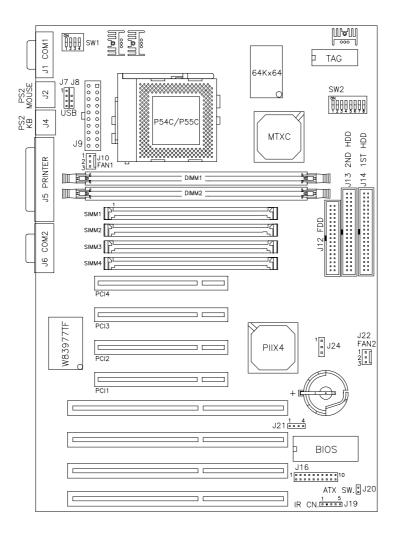
Figure 1: Layout of the TI5TT Motherboard
