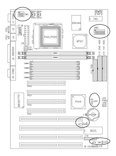
**Figure 2: Jumper Location of the TI5TT**
