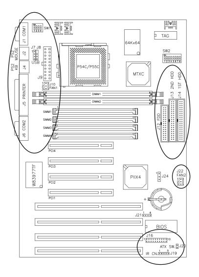
Figure 3: Connector Locations of the TI5TT
