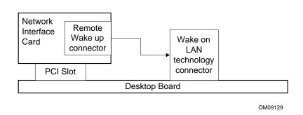
Figure 4. Using the Wake on LAN Technology Connector
