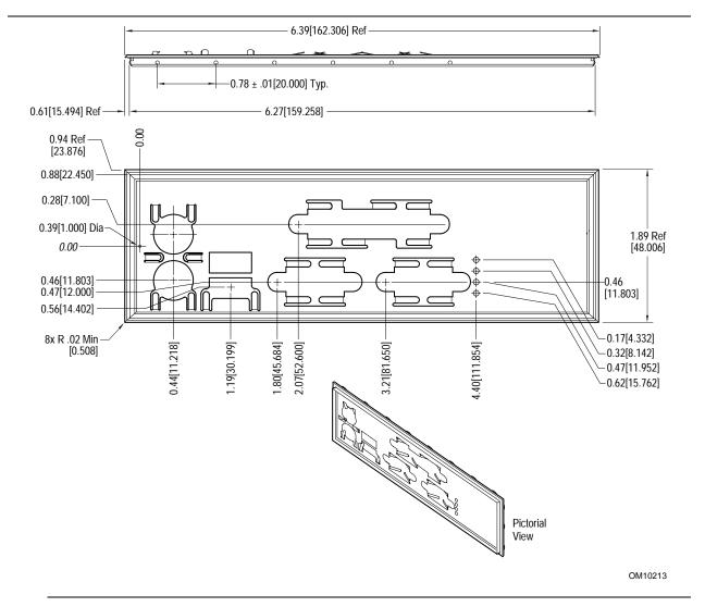
Figure 12. I/O Shield Dimensions
