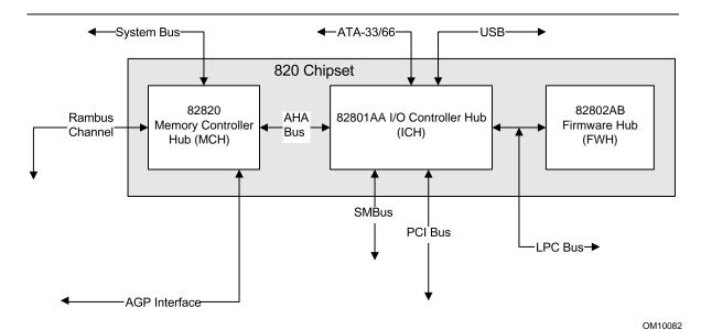
Figure 3. Intel 820 Chipset Block Diagram
