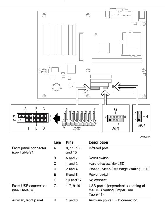
**Figure 9. Front Panel Connectors**
