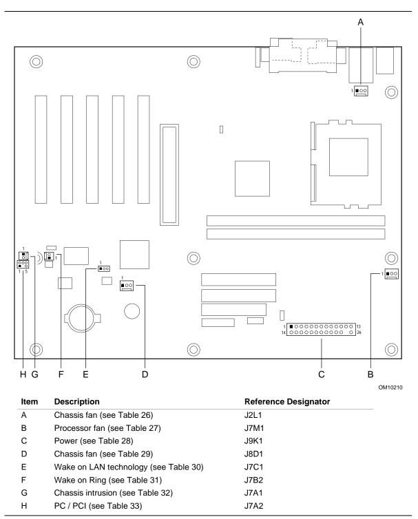
Figure 8. Hardware Control and Power Connectors
