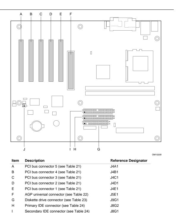
Figure 7. Peripheral Interface and Add-in Board Connectors
