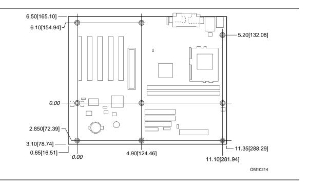
Figure 11. D820LP Board Dimensions
