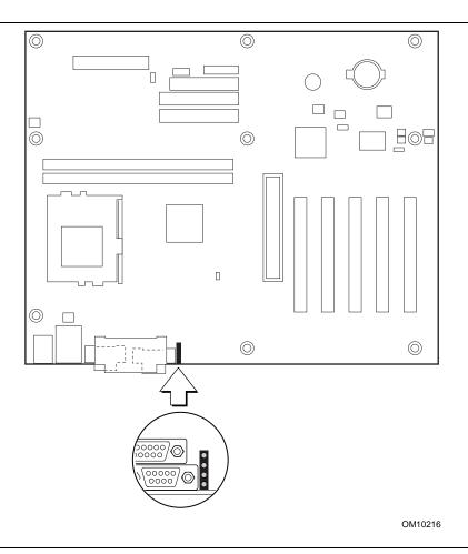
Figure 15. Enhanced Diagnostic LEDs
