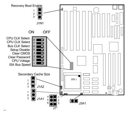
Figure B-1. Switch and Jumper locations (default settings shown) - \*Denotes jumper block found only on PBA 647633
