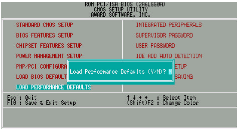
Figure 4.8: Load Performance Defaults
