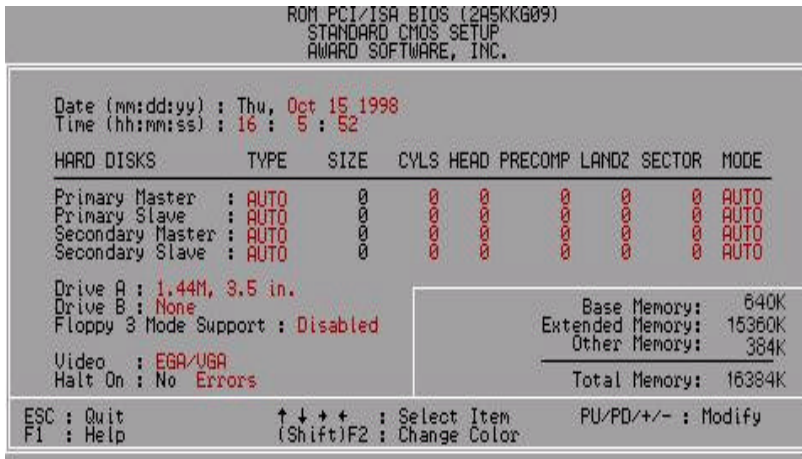
Figure 4.2: Standard CMOS Setup Menu
