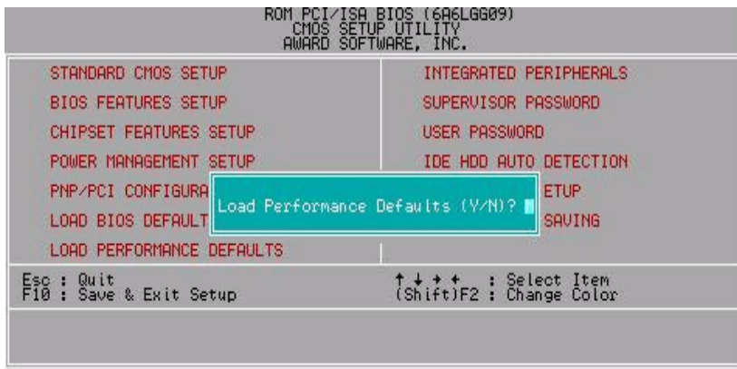
Figure 4.8: Load Performance Defaults
