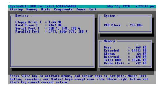
**Figure 3-1** System Configuration Utility (SCU)
