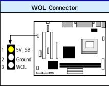
In order to use the WOL LAN card or the modem to trigger the power on the PC system, the switching power supply must have the ability to provide a driving current of at least 720 mA and be connected to a "5V standby" voltage.
