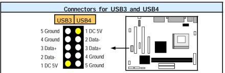
Note: These are not the standard USB connectors you find on the ATX PC99 connector. To connect USB devices you need to use an expansion cable (purchased separately) that ends in a standard USB connector. Ask your retailer for more details.
