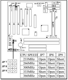
JP7, JP8 and JP9 are used to select the clock ratio for the CPU. Please refer to the figure above for the setting of clock ratio.
