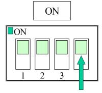
Push the switch upward to select "ON"
