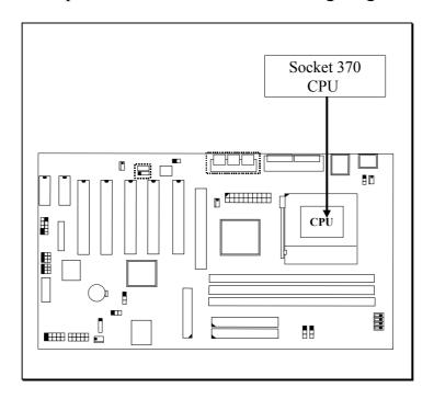
When you have installed the processor onto the mainboard, it will detect the CPU type and decide the CPU voltage automatically. So you don't have to make any jumper setting to select the CPU voltage and CPU FSB clock. If you want to choose other FSB clock and Vcore, please refer to Section 4-11 for the detail.
