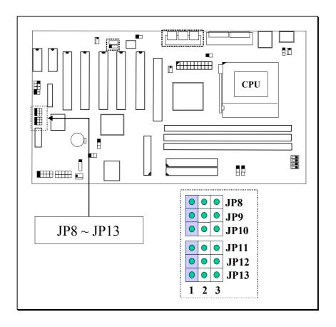
JP8  $\sim$  JP10 are used to control the resource between USB3 (CN30) and CNR1. Following is the details:
