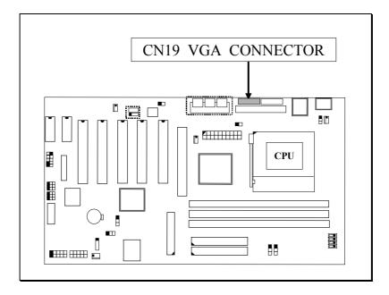
The VGA connector on the board is the AGP VGA interface and you can connect it direct to your VGA monitor. Be sure to refer to Section 3-5 to install the device driver so that the onboard VGA interface can be recognized by the operation system.
