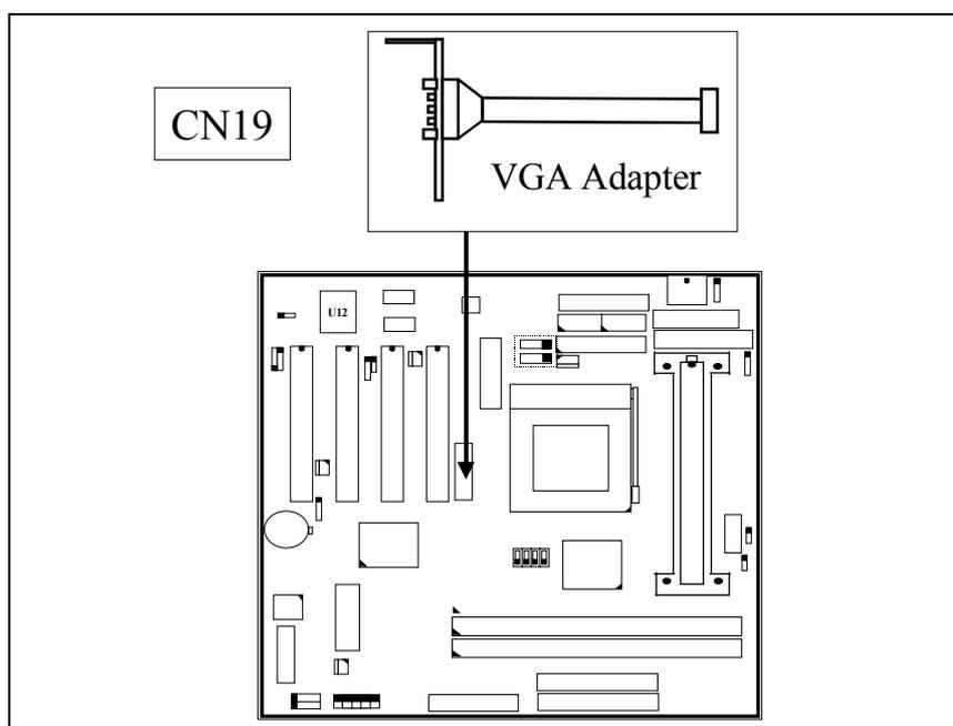
The VGA connector on the board is the AGP VGA interface and you can use an adapter as shown in the above picture to connect it to your VGA monitor.
