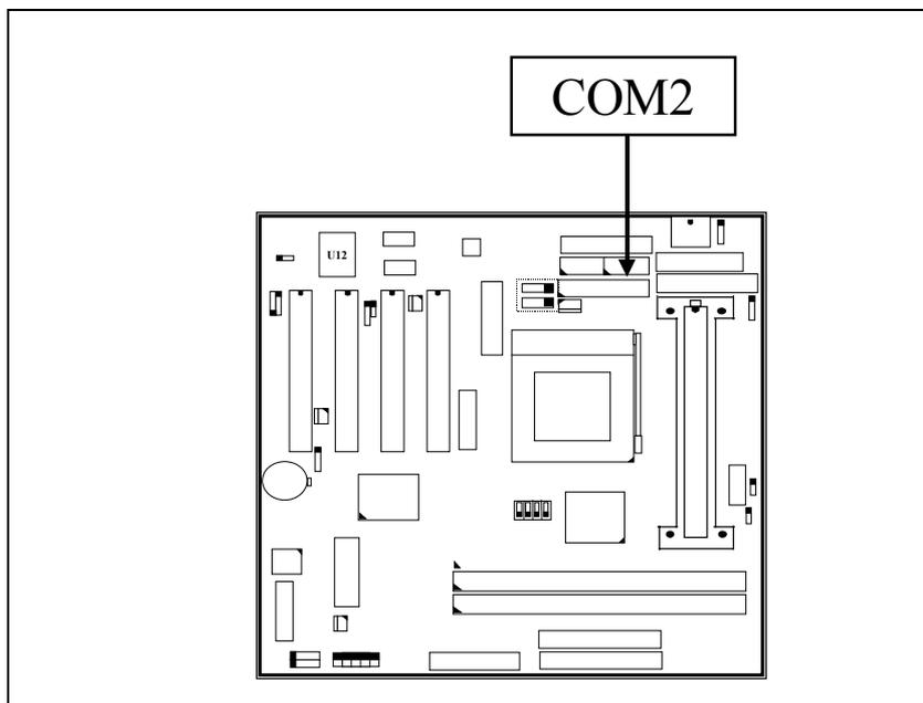
I/O address 3F8H/2F8H/3E8H/2E8H, IRQ3/IRQ4, selected by CMOS setup.
