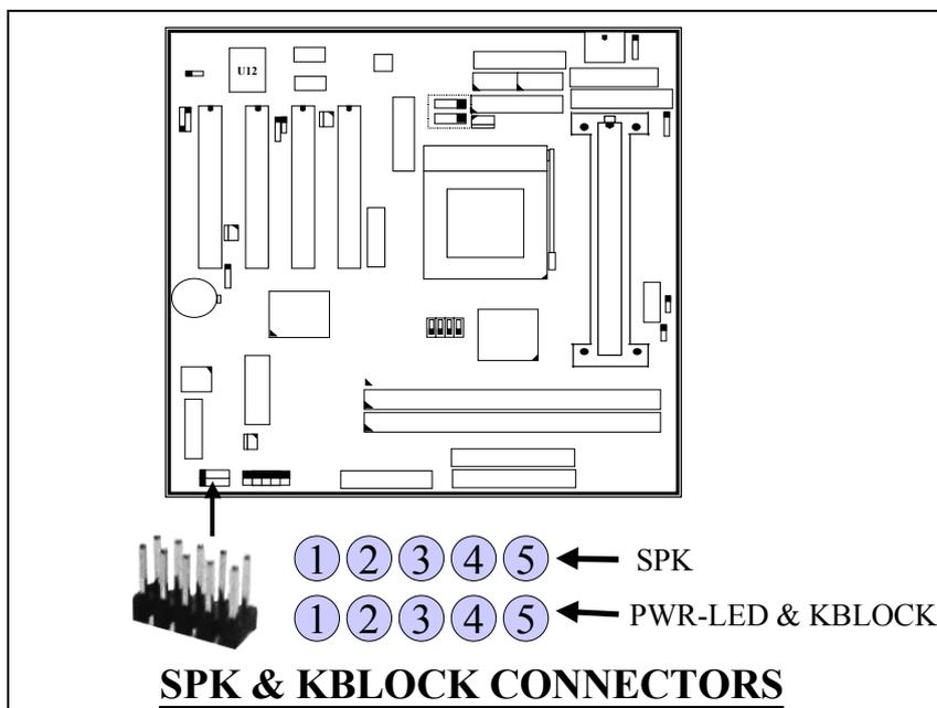
PIN ASSIGNMENT OF SPK CONNECTOR:
