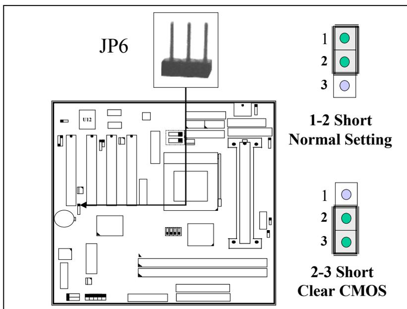
*Note: Improper BIOS setting may cause hang-up to the PC system, Should it be happened, you may use JP6 to clear the information which is stored in the CMOS memory and get the PC system back to normal. Improper connection may cause permanent damage to the mainboard. Please refer to the following steps to clear the CMOS*
