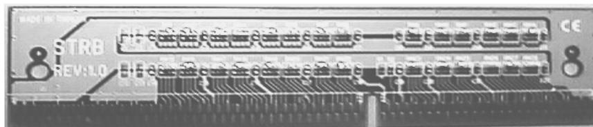
*Install the CPU booster on Slot 1 allows you to use the 133MHz FSB CPU on socket 370 and it will increase the system performance.*
