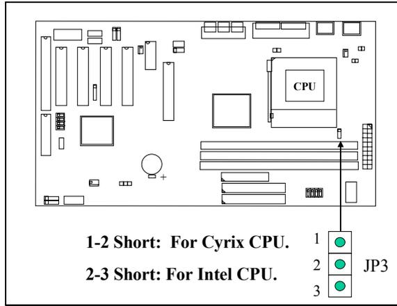
JP3 is disabled and it is not installed on the mainboard.
