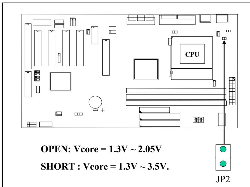
*When JP2 is not installed on the mainboard, it will support Vcore between 1.3V and 2.05V.*
