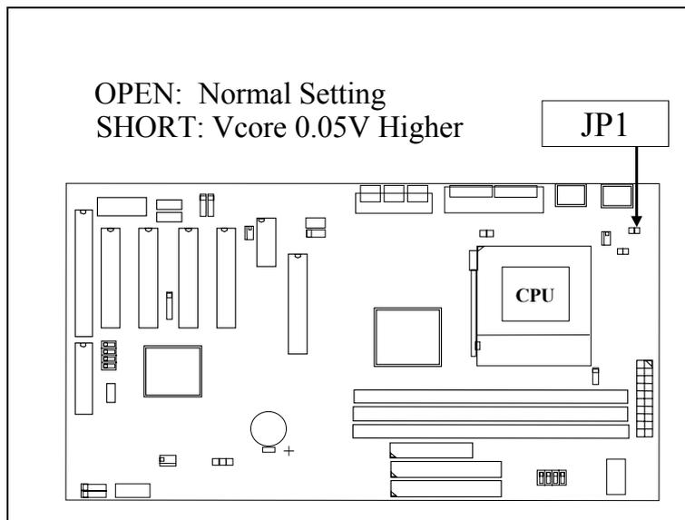
**Note: When you use JP1 to raise the CPU voltage, it does not mean that CPU over clock is guaranteed!.**
