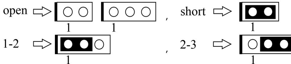
A jumper is a set of two, three or more jumper pins which allow users to make different system configuration by putting the plastic connector plug (mini-jumper) on it. The jumper setting is necessary when installing different components onto the mainboard.
