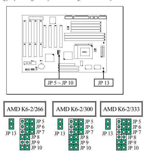
**NOTE**: JP13 is designed to support the 2.2V CPU Core voltage, When short connected, the CPU Vcore will be 2.2V and it will allow you to install the AMD K6-2 processors. If you are not using the AMD K6-2 processors, please leave JP13 open and refer to the manual for jumper settings.
