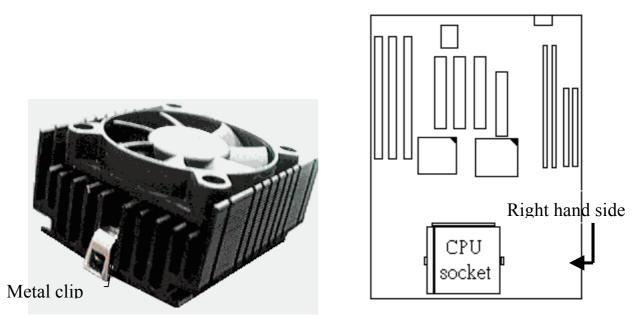
2.Place the CPU cooler squarely on the top of CPU.
