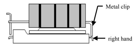
3. Hook the right hand side clip to the CPU socket first.
