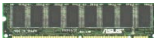
SDRAM DIMM (8 chips, Non-ECC)
