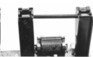
One retention mechanism with brace bar installed
